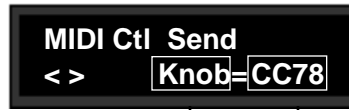
Two fields are available for mapping MPX G2 controls to MIDI controllers.
